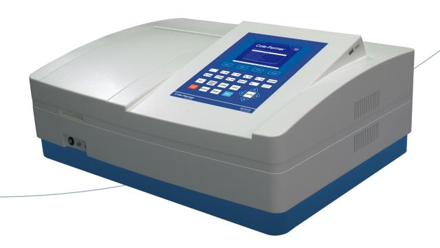
The SP-800-UV is a UV-Visible double-beam spectrophotometer with a variable spectral bandwidth. The spectrophotometer has an integrated user interface for local control and ease of navigation. The highly stable optics and two detectors measure the sample and reference simultaneously, optimizing measurement accuracy.
